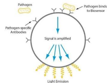
The Zephyr Pathogen Identifier uses CANARY® detection technology to screen for pathogens in liquid and powder samples. The Zephyr platform is ideal for users who need rapid, accurate results, and who test lower volumes of samples (<40 tests/day).
